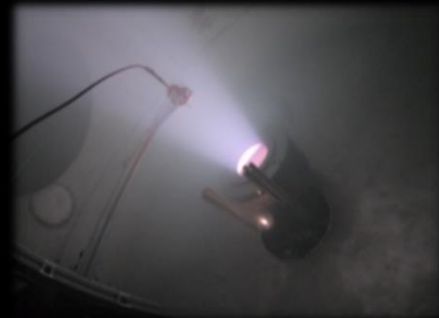
12 cm plasma source operating at MST [Folta, B. (2020)]
